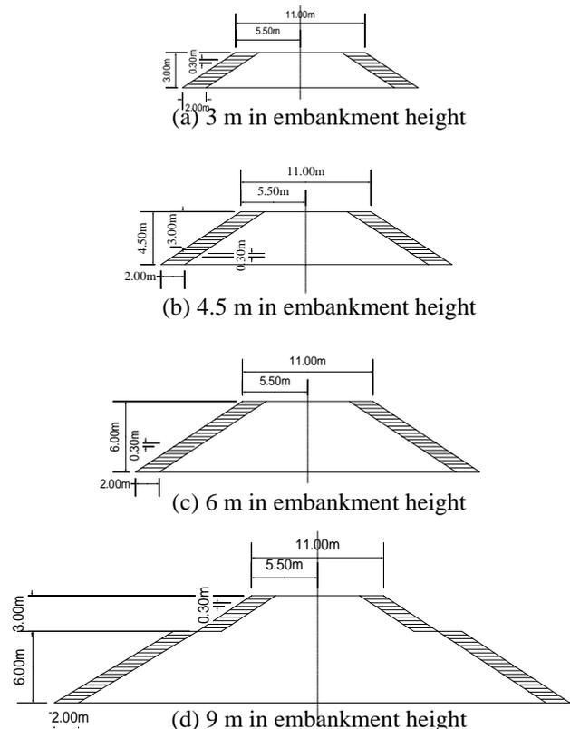
Figure 2. Cross sections of embankments (Performance rank II and III, gradient of slopes 1:1.5)
