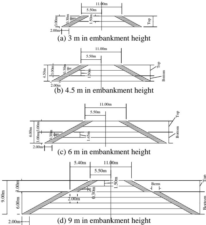
Figure 1. Cross sections of embankments (Performance rank I, gradient of slopes 1:1.8)
