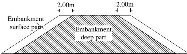
Figure 3. Division of embankment surface and subsurface
