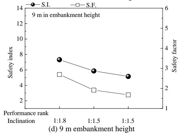
Figure 6. Performance rank versus safety index and limit state exceedance probability
