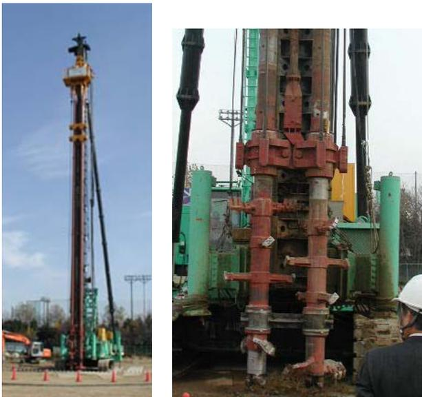
Figure 1. In-situ mechanical mixing machine using cement-slurry
